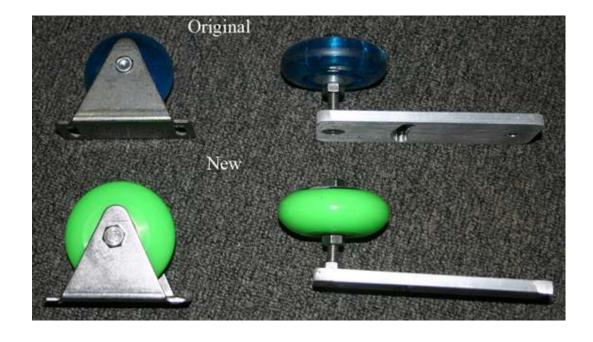
What I use was 20 new 59mm rollers, 40 zero drag 608 bearings, 20 6mm bearing spacers, 10 SS  $1/4 \times 20 \times 1 \times 1/2$ " bolts, 20 SS 1/4" washers (to space out the wheels on the base rollers one on each side), and 10 SS 1/4" acorn nuts.
