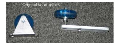
I drilled out the side that was flared out to remove the pin. After drilling the head off I use a punch to drive out the pin and that allowed me to take the roller assembly apart.
